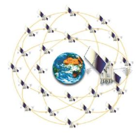
The GPS (Global Positioning System) is a radio navigation system, which lets you know exactly where you are on the globe, in three dimensions. Moreover, this information is available 24 hours a day, and in any weather conditions. This system features 24 satellites and a monitoring network, which are financed and operated by the US Department of Defence. One part of this system is reserved for military purposes, while the other part can be used by anybody for free.
