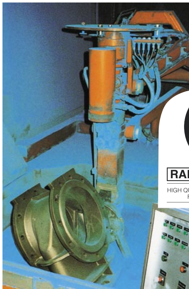
Fluidised bed Epoxy powder coating at 200° C
